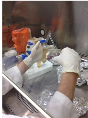
Place into B. staerothermophilus ( 2.7 \times 10^6 cfu/ml) in trypticase soy broth- Day 1
